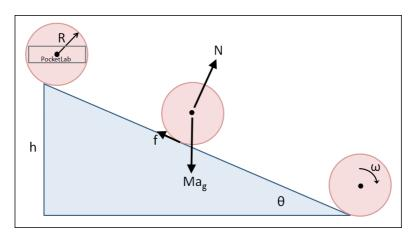
We will use conservation of energy to determine the velocity of the cylinder at the bottom of the incline, though this can also be done from the use of dynamics as well. While rolling down the incline, the cylinder loses  $Ma_gh$  of potential energy. Meanwhile, it has gained an amount of kinetic energy equal to
